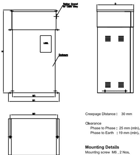
Drawing 2 - Three Phase, Rectangular Capacitor Bank
